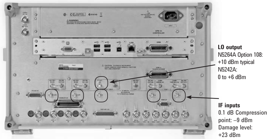
Figure 23. PNA-X N5242A network analyzer and PNA-X N5264A measurement receiver rear connectors.
