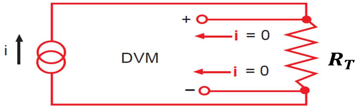
4-WIRE OHMS MEASUREMENT
