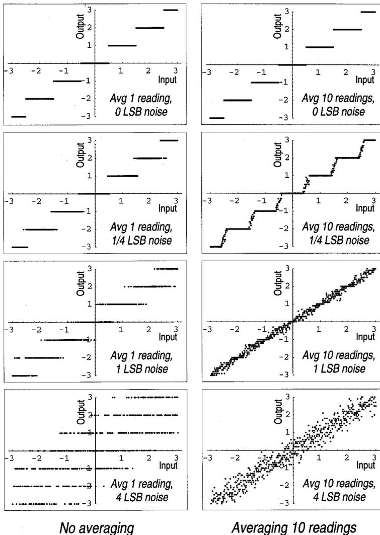
FIG. 2. A/D output with 0, 1/4, 1, and 4 LSB of noise added to the input, with no averaging (left side) and with each data point the average of 10 readings (right side). Scales are in LSBs.
