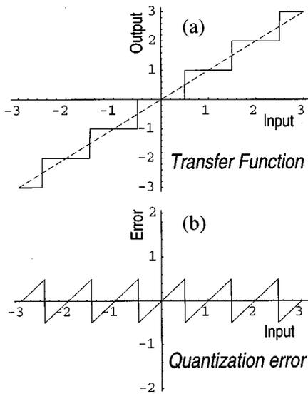
FIG. 1. Transfer function (a) and quantization error (b) for a hypothetical A/D converter. Units are in LSBs.
