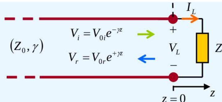
$$\left. \begin{aligned} V_L &= V_{0i} + V_{0r} \\ V_L &= \frac{Z_L}{Z_0} (V_{0i} - V_{0r}) \end{aligned} \right\} V_{0i} + V_{0r} = \frac{Z_L}{Z_0} (V_{0i} - V_{0r})$$
