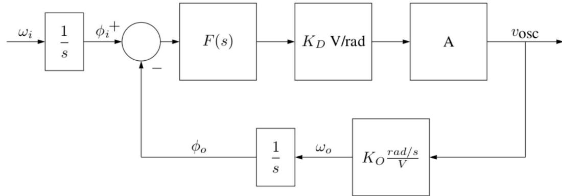
$$\frac{V_{\text{osc}}(s)}{\Omega_i(s)} = \frac{K_D A F(s)}{s + K_D A F(s) K_o}$$
